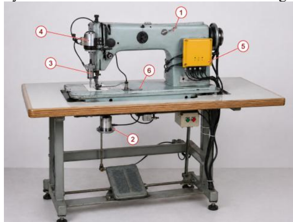
Fig. 1. Experimental platform of the integrated ultrasonic-assisted sewing system. The conventional sewing machine is integrated with the ultrasonic modules for fabric feeding, needle penetration and thread-tension regulation, along with the corresponding control and power-supply units: 1 — needle/penetration zone; 2 — drive and support frame; 3 — fabric-feeding area; 4 — sewing machine head; 5 — ultrasonic generator/control unit; 6 — working table and material support area.
