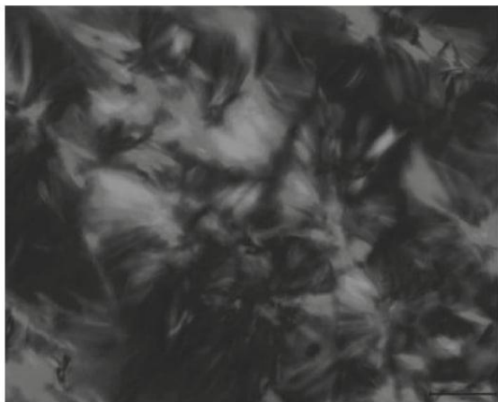
Appearance of DF paraffin crystal morphology using BX41-P OLYMPUS polarizing microscope.
