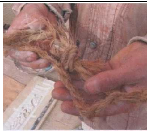
Fig. 5.2 Sazu, the traditional rope used for hanging layers of muqarnas (Source: Hamidreza Kazempour)
