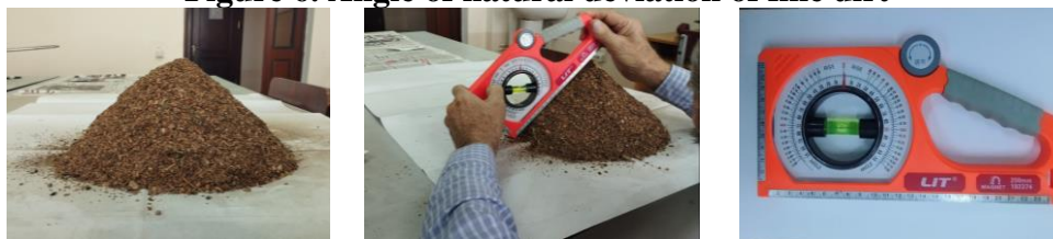
Figure 6. Angle of natural deviation of fine dirt
