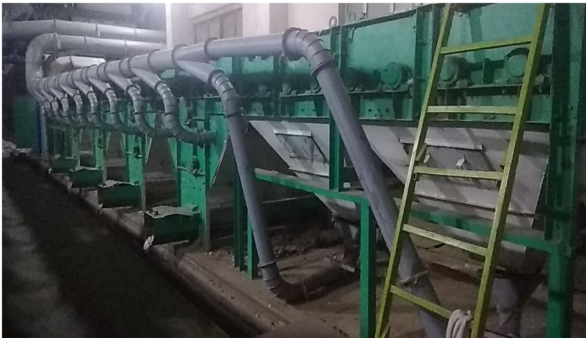
Figure 2. Overview of the aspiration system
