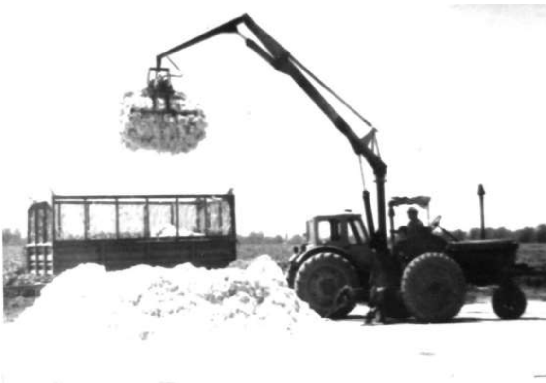
Fig.4. Work of a loader with an experimental grapple on loading raw cotton into a trailer.
