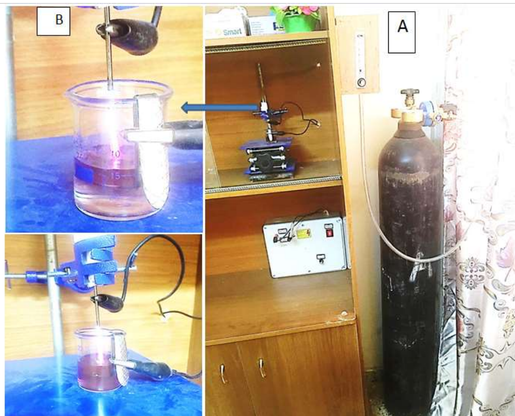
Figure 1 illustrates the plasma system generating nanomaterials(a) Connecting the system with the argon generator (B) illustrates plasma generation to produce nanomaterials.
