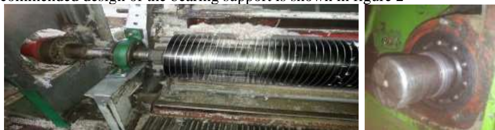
Fig 2. Prototype of a bearing with an elastic element (2 different thicknesses) mounted on the saw cylinder shaft.
