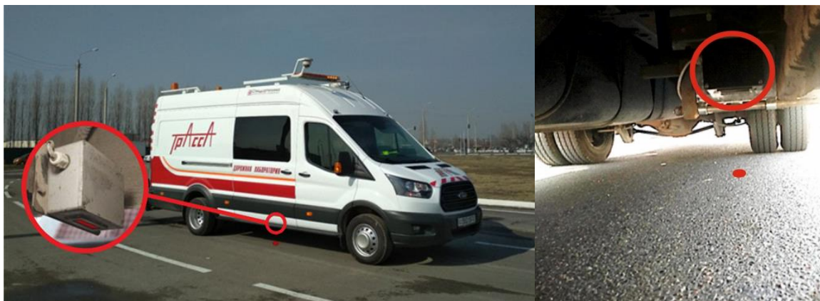
Fig 2. The IRI system for measuring the road roughness and operation of the PKR-2 laser profilometer at the MRL “Trassa”
