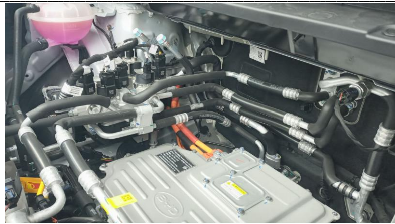
Figure 7. Location of thermal management system pipelines
