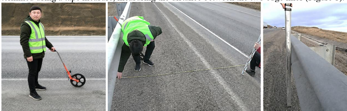
Figure 1. The process of measuring the longitudinal slope of the road and the width of the roadway.
