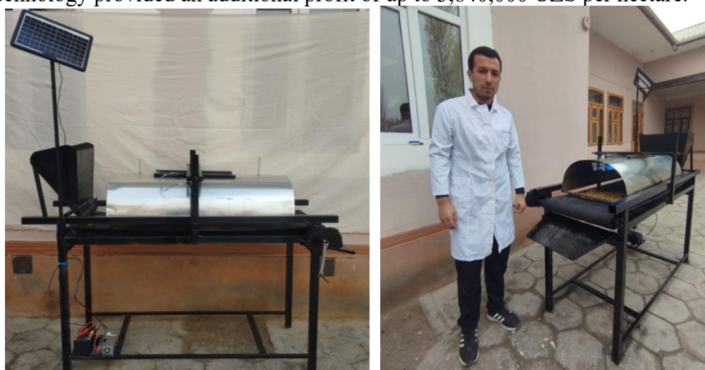
Figure 3. Device for ultraviolet treatment of seeds
