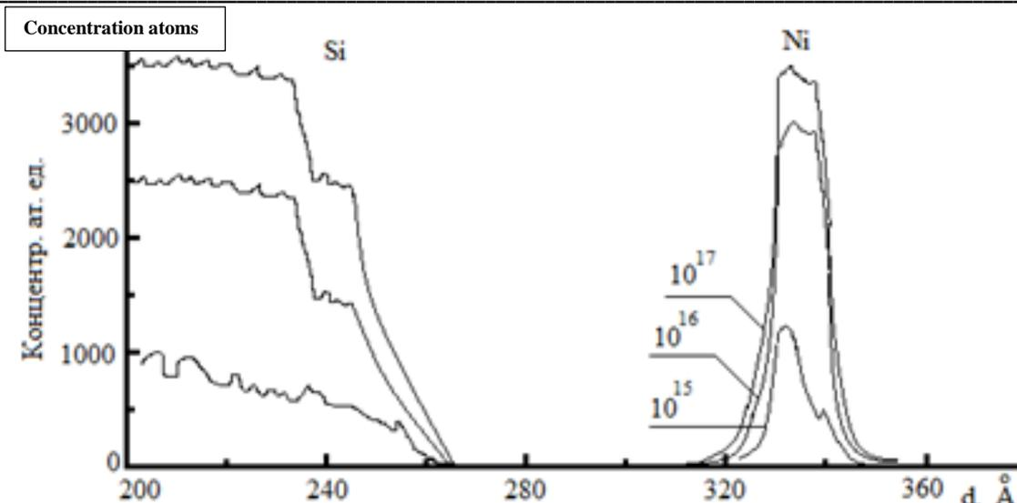
Figure2. RBS spectra of  $\text{He}^+$  ions on a single crystal of Si doped with 40 keV Ni ions with doses of  $10^{15} \div 10^{17}$  ion/cm<sup>2</sup>
