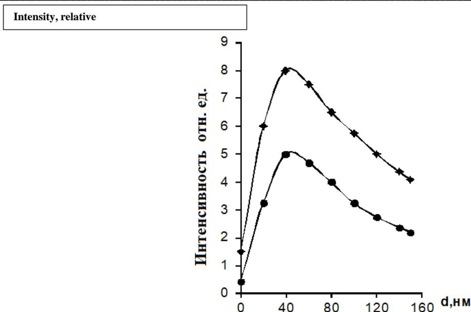
Figure 3. The distribution profiles of doped Ni atoms in Si doped with a dose of  $10^{16} \div 10^{17}$  ion/t/cm<sup>2</sup> obtained by the VIMS method.
