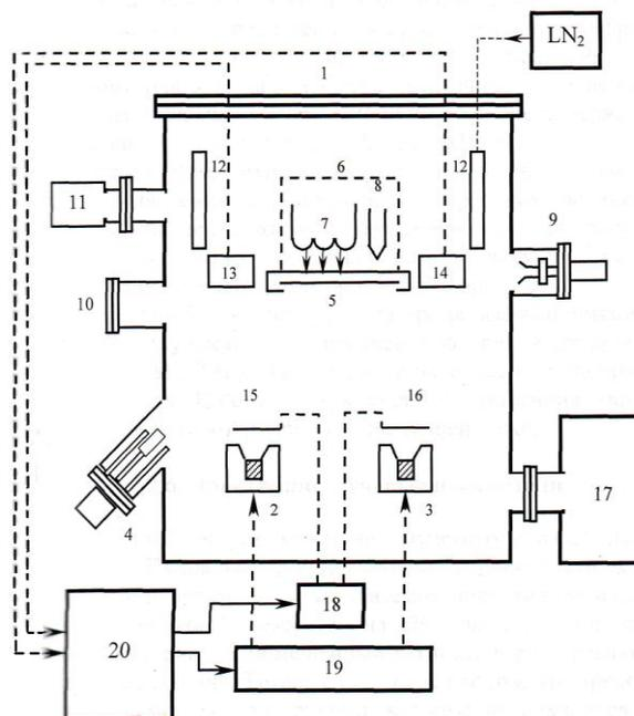
Figure 1. Analytical growth chamber 1, 2, 3 –electron beam evaporators; 4-effusion source; 5 sample; 6-manipulator; 7-heater; 8-thermocouple "9-electron gun of a fast electron diffractometer; 10 luminescent screen; 11 quadrupole gas analyzer; 12 cryostat panel; 13,14-quartz deposition rate sensors; 15,16-flaps; 17-ion pump; 18-control valves with thermal; 19 power supplies for electron beam evaporators; 20 computer
