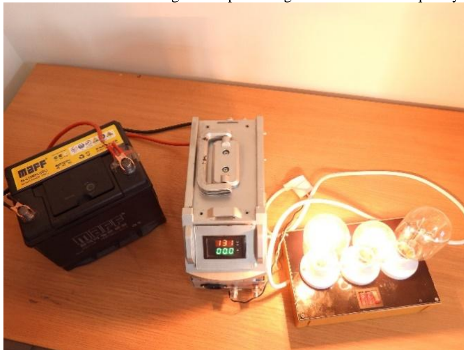
Fig.3. 3KW inverter with a rectangular output voltage of 220V and a frequency of 50 Hz
