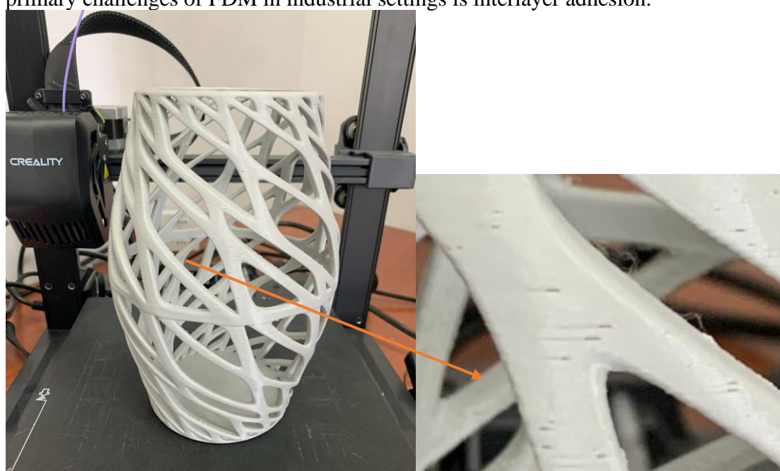
Fig. 1. Examples of printed components with varying interlayer adhesion
