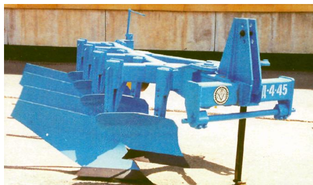
Figure 4. The PD-4-45 two-half four-corpus hanging plug is designed to drive unworn rockless land up to 40 cm in diameter
