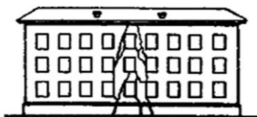
solid foundation weak foundation solid foundation
