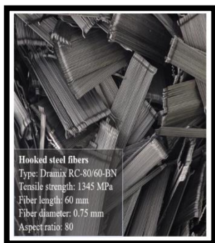
Fig.14 hooked Steel fiber used
