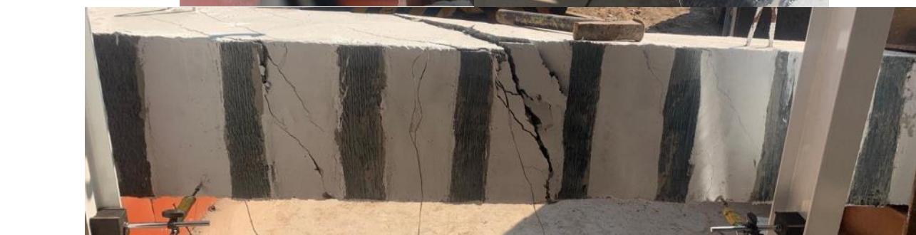
Figure 8: Strengthened beam ES-2 failure and crack configuration.
