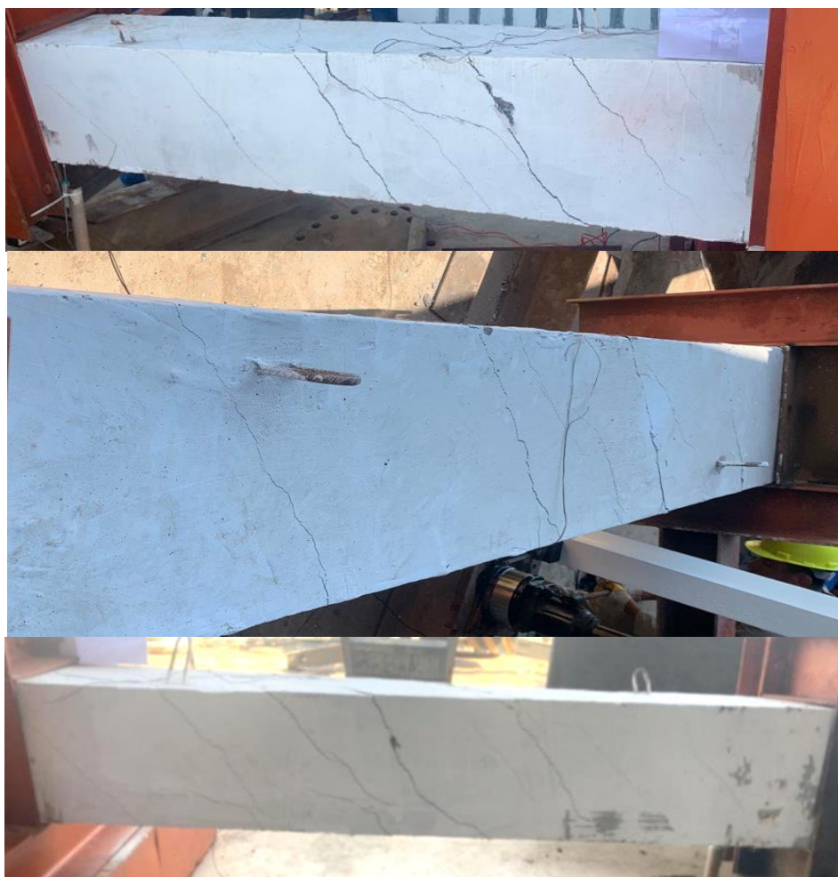
Figure 6: Control beam C-0 and C-1 failure and crack configuration
