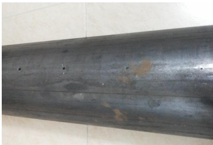
Figure 1-3. Close-up vertical perspective showcasing the pipe and its perforations.
