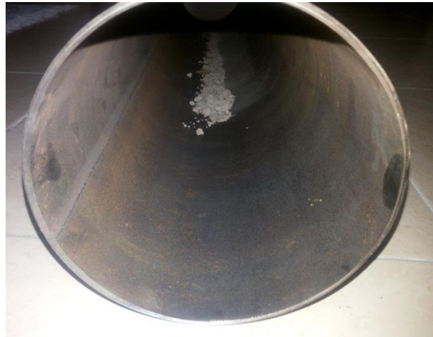
Figure 1-4. Cross-sectional depiction of the pipe, highlighting the internal sediments.
