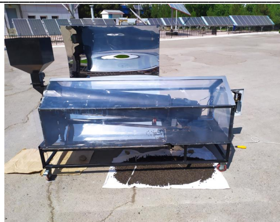
Figure 1. Scheme of combined energy-saving experimental drum dryer: 1-loading hopper, 2-stepper motor for adjusting grain consumption, 3-drying drum, 4-rotating rollers, 5-rotating rollers hardened support, 6-gear wheel fixed on drum, 7-drum rotating motor, 8-electric heater, 9-fan, 10- electric furnace power supply conductor, 11- sensor cables that transmit information about temperatures, 12-control cabinet, 13-parabolic tube reflector, 14-reflector fixed metal profile, 15-solar collector, 16-the metal frame of the solar collector, 17- the lower support part of the dryer, 18-wheels that move the dryer, 19-metal panel blocking the solar collector from the front, 20-metal panel blocking the solar collector from the bottom side, 21-unloading hopper.
