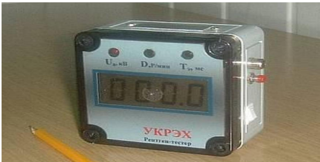
Fig. 1 Device for monitoring radiation and electrical characteristics.
