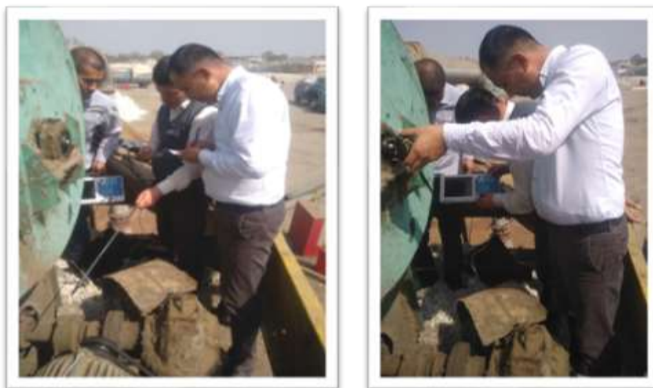
Figure 2. The process of checking the movement of the shafts of the equipment using an oscilloscope
