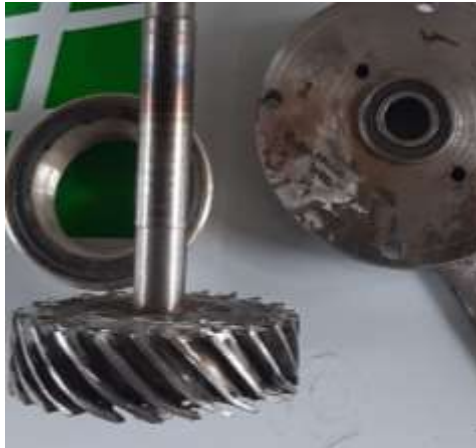
Figure 2. Model of micro-HEP jet hydro turbine working wheels: a) 200 W power; b) with a power of 1 kW;
