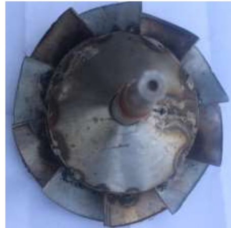
Figure 2. Model of micro-HEP jet hydro turbine working wheels: a) 200 W power; b) with a power of 1 kW;
