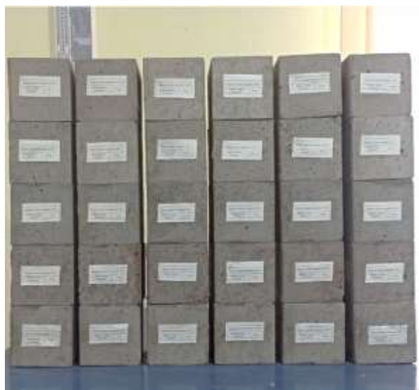
Figure 2. Concrete cube samples with basalt fibers
