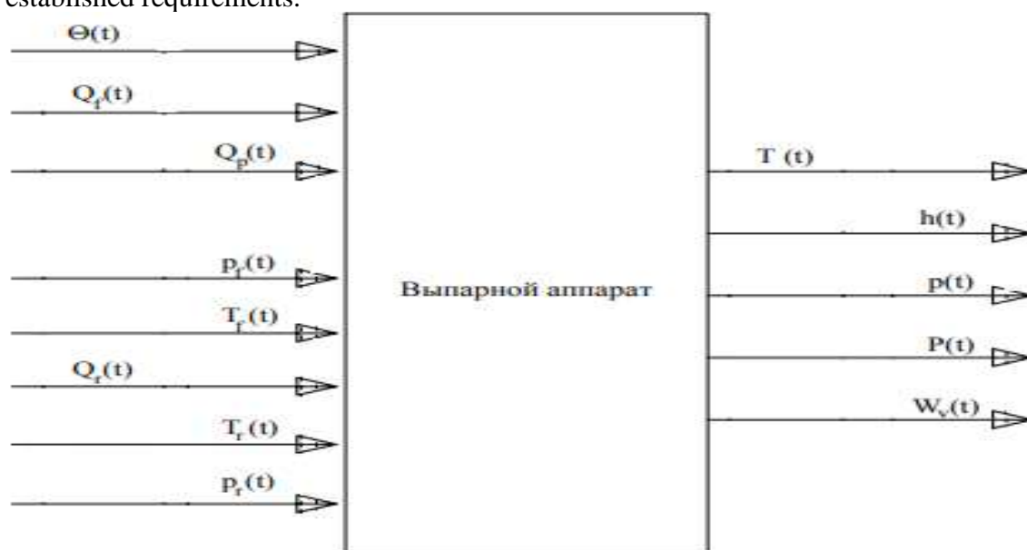
Fig.2. Composition of the main variables of the computer model of the evaporation apparatus
