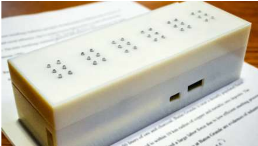
Figure 3. Real-time text to Braille converter
