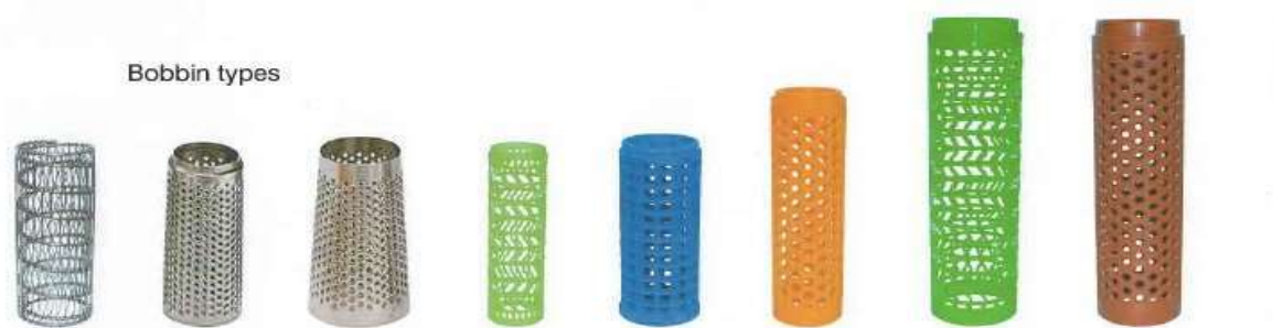
Picture 3. Iron or plastic cartridges used in yarn dyeing.
