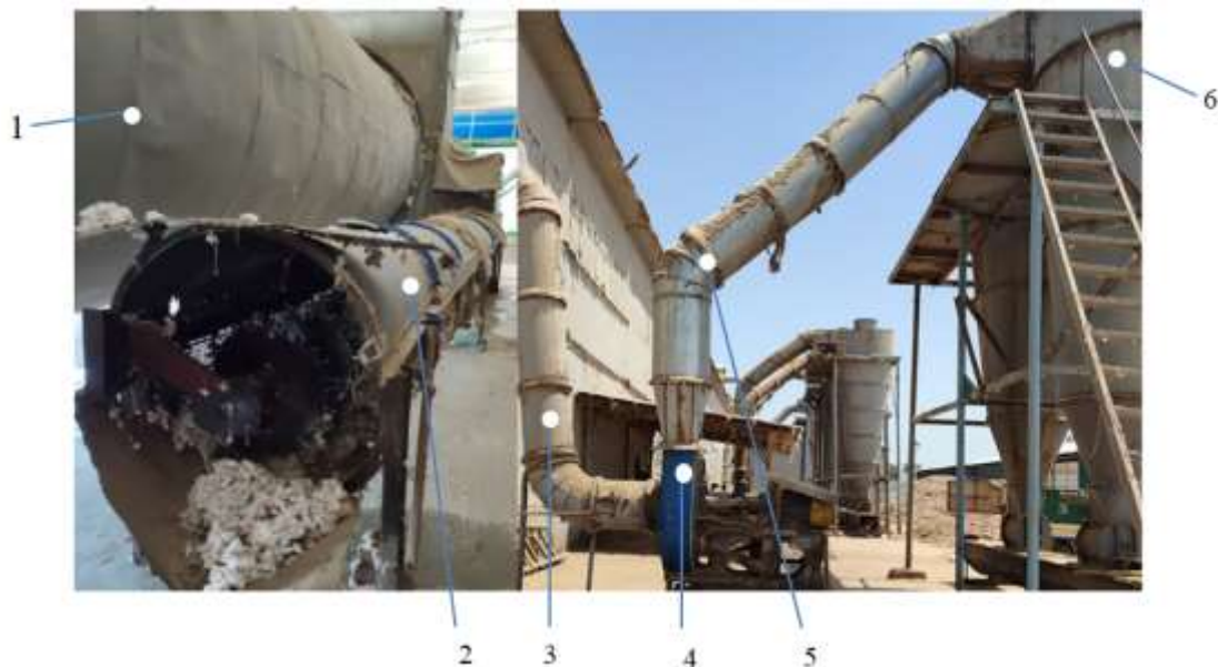
Figure 1. A system of devices for removing particles of fine litter and dust from raw cotton at ginneries. 1-Device for drying cotton (2SB-10); 2-device for cleaning fine dirt and dust from cotton; 3 and 5 pipes; 4-fan (VTs-10M); 6-device for collecting dust (TsS-6).
