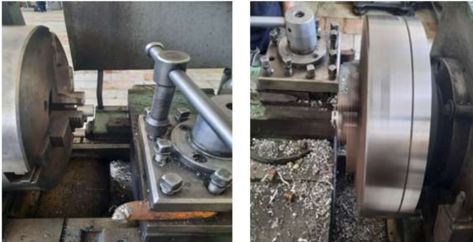
Figure 2. The process of extracting fragments from samples on a lathe.
