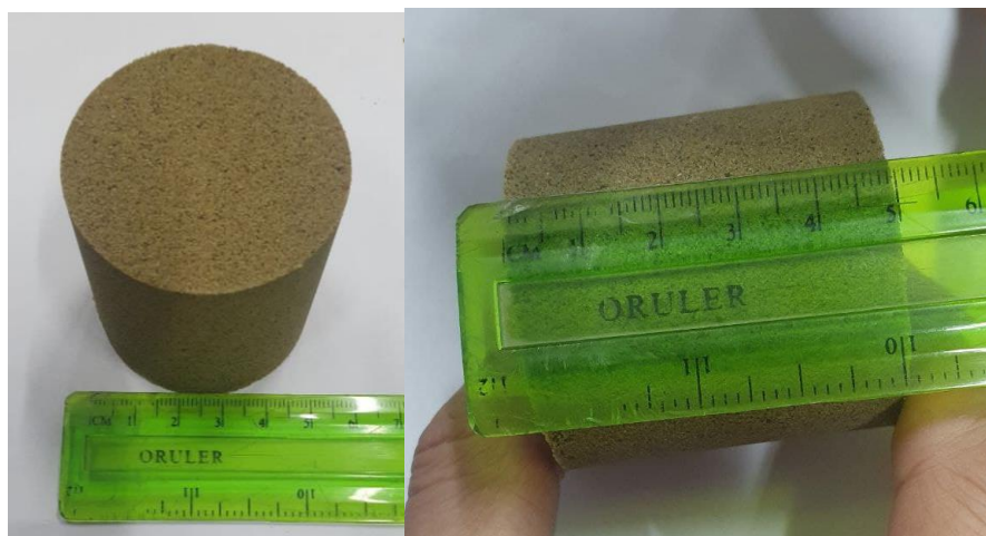
Figure 3 - Test samples with dimensions of 50 x 50 according to GOST 23409-78
