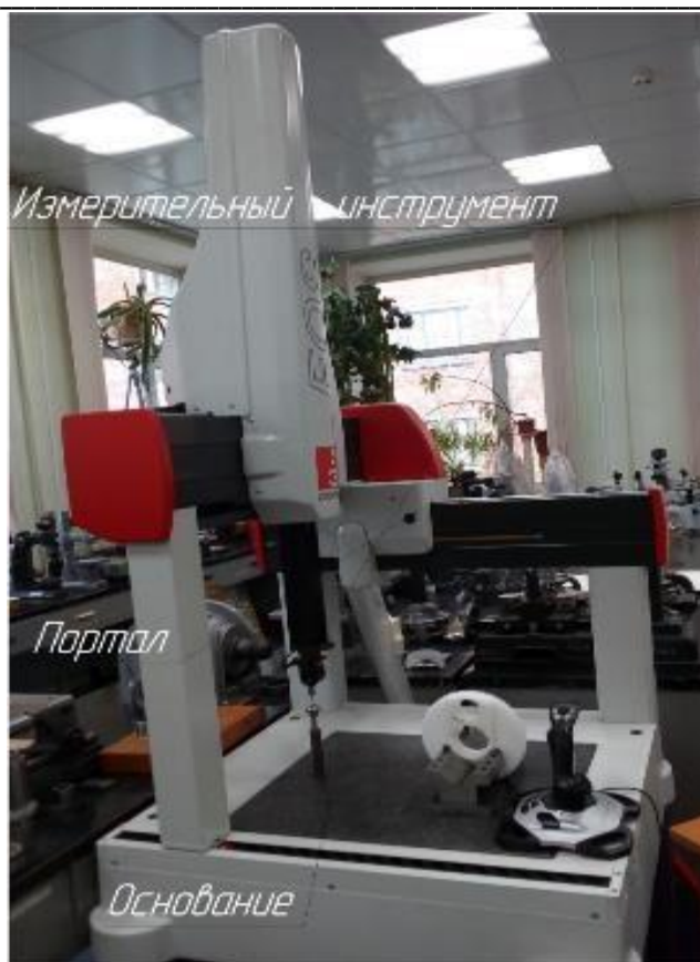
Measuring tool // portal // base Fig. 1. Plate-measuring machine.
