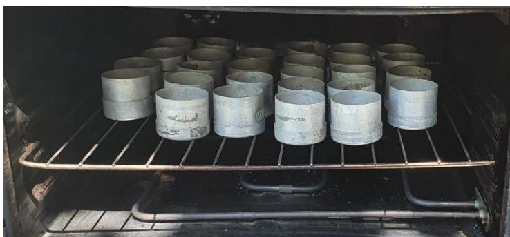
2- picture: Drying soil in a special oven
