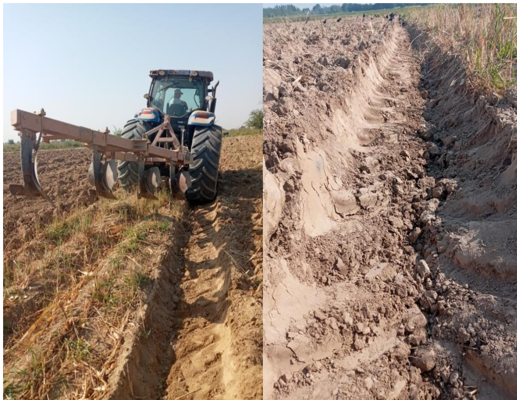
Figure 1. The process of studying compaction by tractor wheels in plowing
